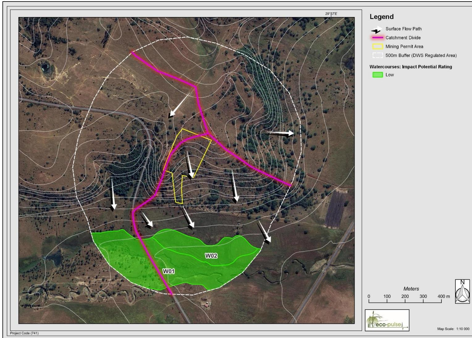
**Figure 4** Outputs of the initial watercourse 'impact potential' assessment undertaken for the mining permit area. The map shows the positioning of the area footprint ("Yellow" boundary line – mining permit area), with watercourses assessed with a 500m radius [i.e., the DWS regulated area for (c) & (i) water use – "white" dashed circle outline].
